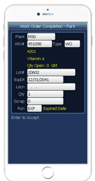
This transaction completes the work order by increasing inventory for the manufactured items and updating the status of the work order to identify it as being complete.
